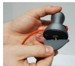
Figure 1: Attach Wetted Cotton Electrode to Puck
