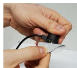
Figure 2: Attach Gel Electrode to Neutral Lead
